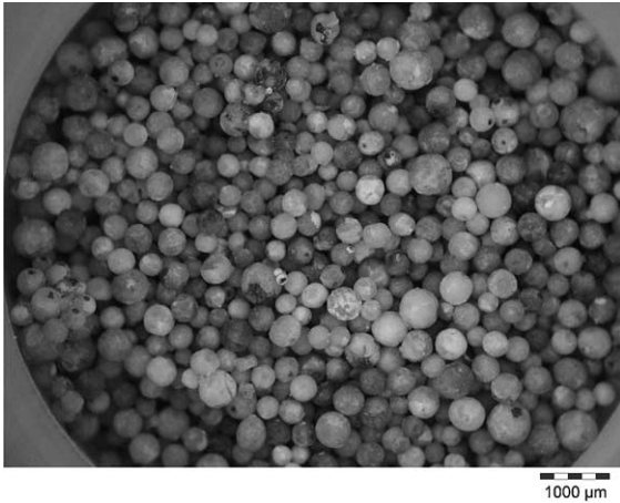
Fig. 2. Overview of irradiated OSi pebbles as delivered at FZK (E8/8-13: outer bed, about 11% burn-up).
